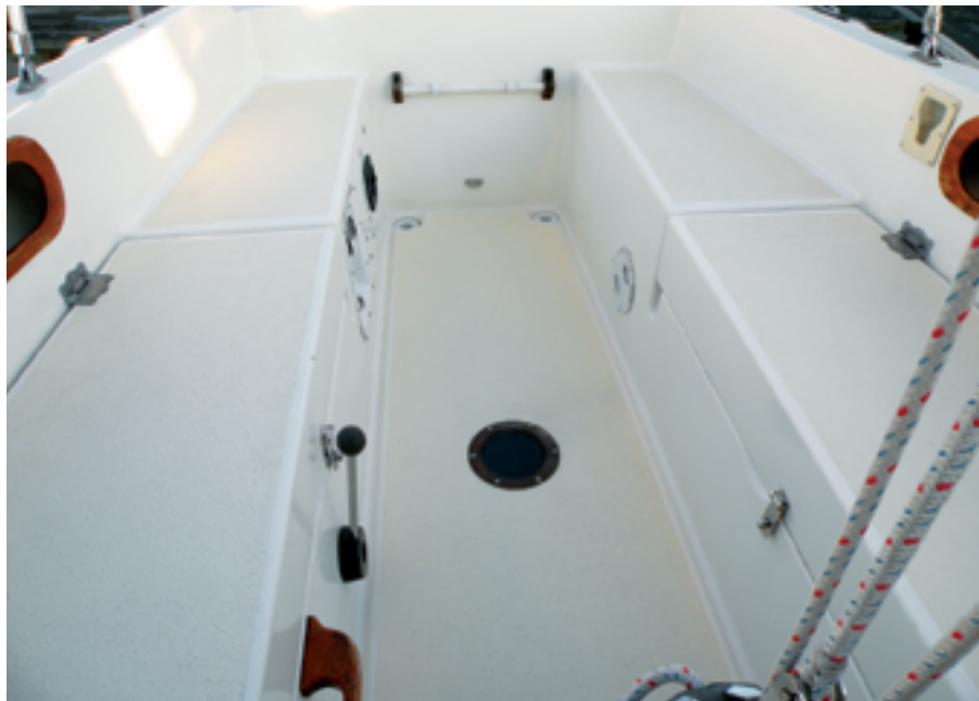
Indecision's cockpit provided ideal surfaces on which to test the non-skid paint.
